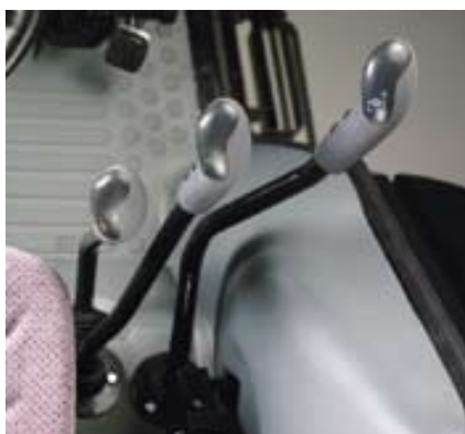
Gear levers from right-to-left: forward/reverse shuttle, four-speed main gear selector, and selector for intermediate ratios.
