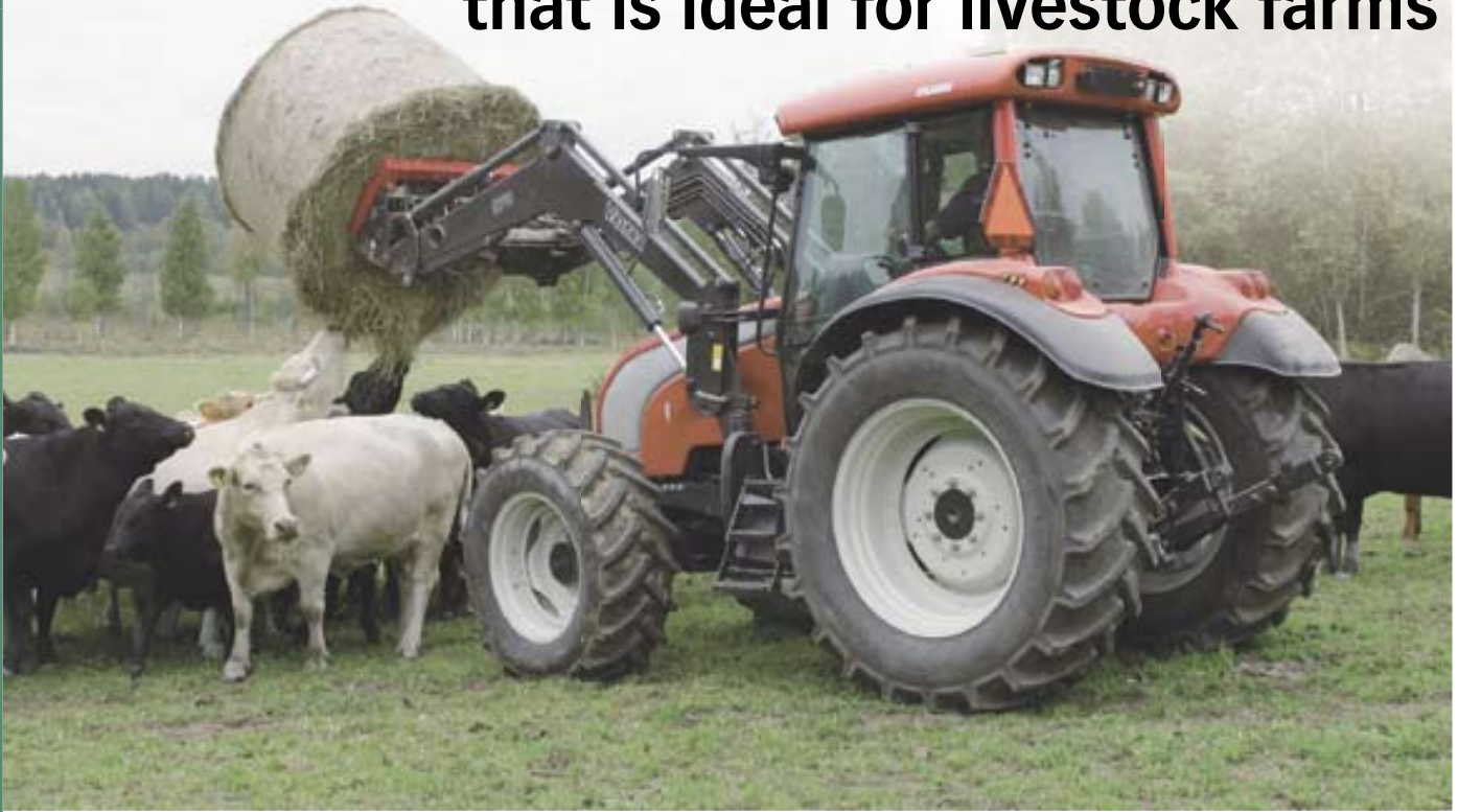
The weight distribution of the C series is 39/61%, which is ideal for front-loader work.
