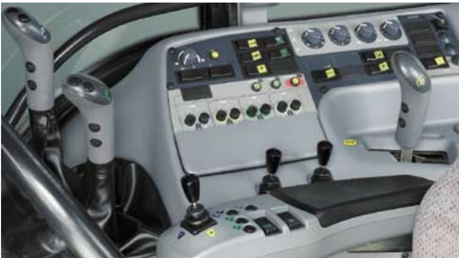
Sauer-Danfoss is a supplier of steering valve for all Valtra models. For the new Valtra M and T series Sauer-Danfoss supply hydraulic valves and Joystick.
