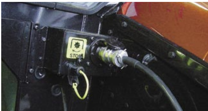
ISOBUS implement is connected by one cable to tractors connector.
