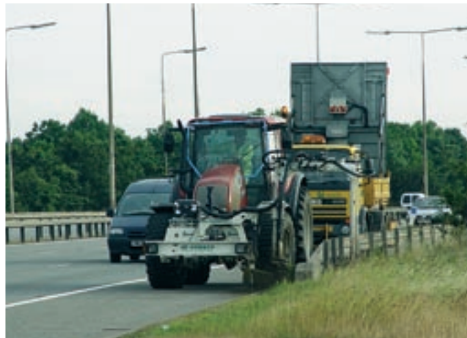
Ian White's front mounted over barrier mower is easy to operate in the dangerous environment of a motorway hard shoulder while a 50 kph transmission makes moving from site to site quick and safer.
